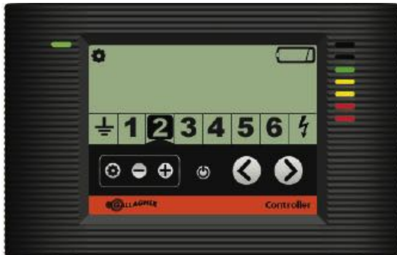
Controller showing zone 2 with a low battery
