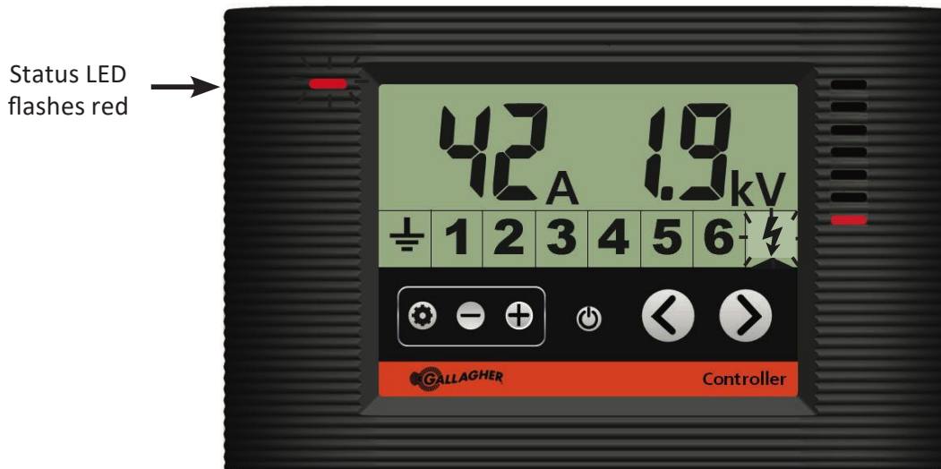
Controller showing the energizer in current alarm
