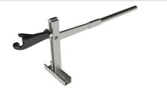
**Line Post Lifter Attachment** G52701 Attaches to most Steel Post Lifters to safely pull out the Insulated Line Post.
