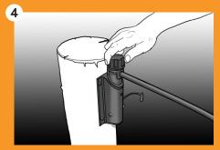
Replace the cap and screw down tightly to lock the rod in position.
