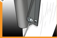
Connect the live wire from the fence to the terminal screw on the side of the hinge barrel using insulated cable.
