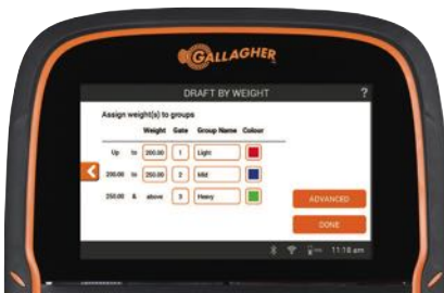
Draft by weight, weight gain or eid list (and traits on the TWR-5 & TW-3)
